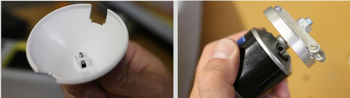
**Left:** plastic spinner removed. **Right:** Motor removed with propeller hub still attached.
