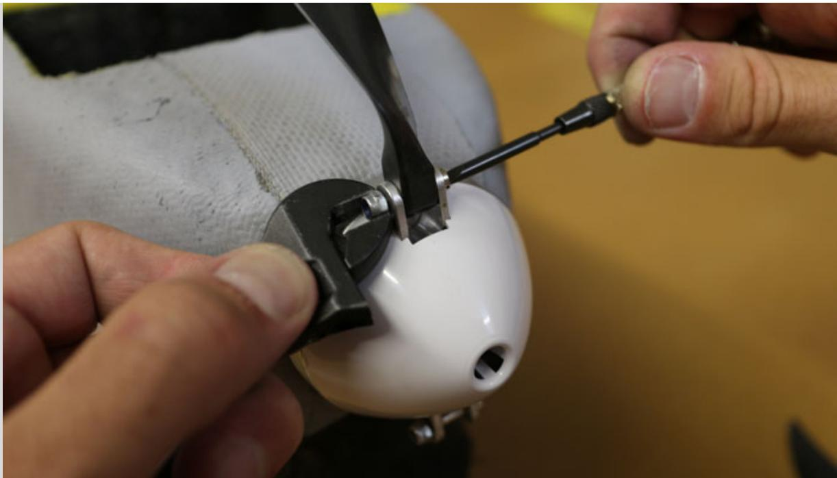
*Remove a propeller using the crescent wrench and flathead screwdriver.*
