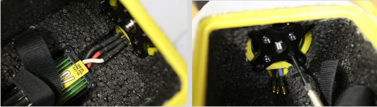
**Left:** Looking into the battery bay. The ESC and motor connect with three wires. **Right:** Four counter-sunk screws fasten the motor to the bulkhead.
