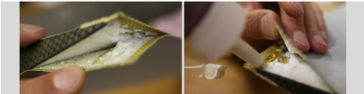
**Left:** Kevlar skin pulled back exposing wing foam. **Right:** Gorilla Glue being applied beneath the Kevlar.
