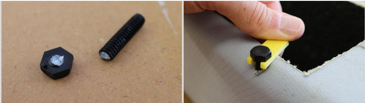
**Left:** Broken wing bolt removed. The bolt will typically shear at the base of the hex cap. **Right:** Wing bolt spacer.
